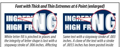
Same text with a stayaway stroke of .003 inches. A clone of the text with a stroke of .0055 inches has been pasted inside the letters. Legibility is improved but not perfect. "G" is still pinched inside. Total stayaway is .00425 inches.
